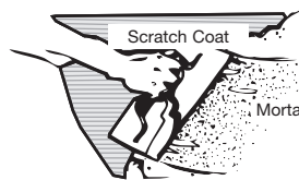
Figure 5 Apply mortar using a plasterer's trowel.
